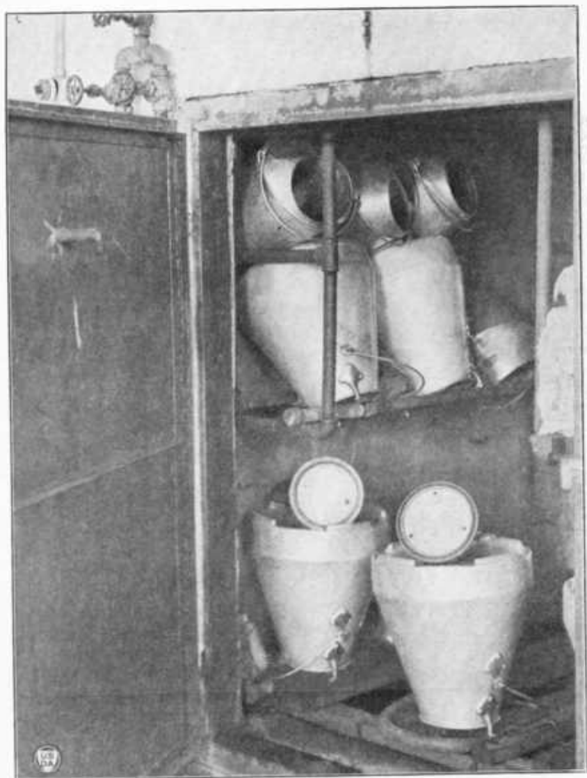
FIGURE 10.—Milking-machine pails and covers should be treated with steam or a chlorine solution. Pulsators and electric motor should be removed before such treatment
